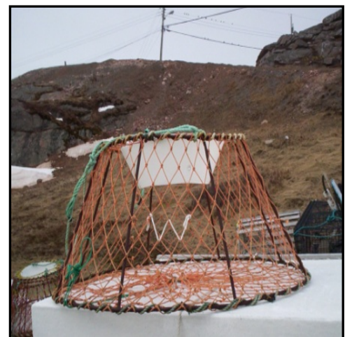
Figure 4.3: A crab pot fitted with biodegradable twine. Note the W shape of the white twine. (Photo Source: Helen Woodrow)
