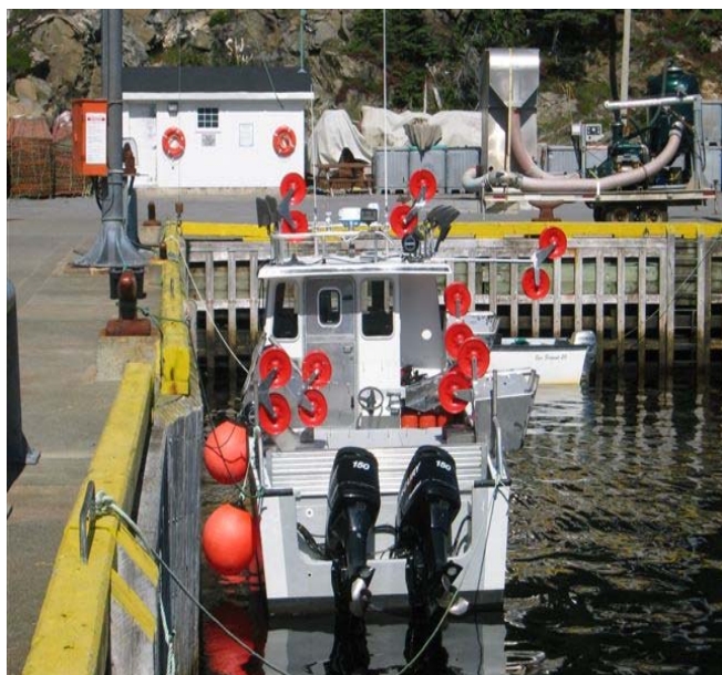
Figure 3.2: Fishing Boat with Pulley and Stripper Systems. (Photo Source: Albert Wells)
